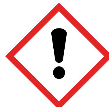
Acute toxicity: Harmful (if swallowed, in contact with skin or if inhaled) Skin and/or eye irritation 急性毒性: 有害 (如不慎吞食、皮肤接触或吸入) 皮肤和/或眼睛刺激
