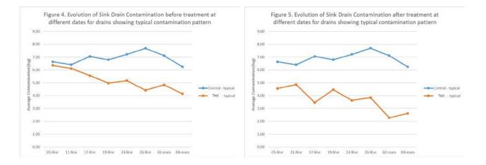
At the end of the trial, the average post-treatment contamination on the Test drains was 2.62 log, which is an average of 420 CFU/swab. At the end of the trial, the average post-treatment contamination on the Control drains was 6.24 log, or an average of 1,750,000 CFU/swab.
